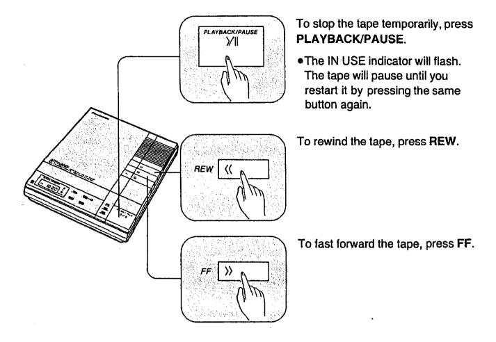
■ If you want the unit to stop rewinding or fast forwarding the tape, press the PLAYBACK/PAUSE button. The unit will play back the tape from the point you press the button.
